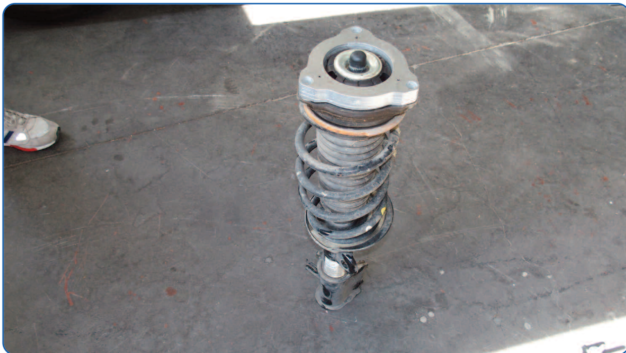
A - Place up to the spring's disk the shock absorber's thickness and let the three holes coincide
