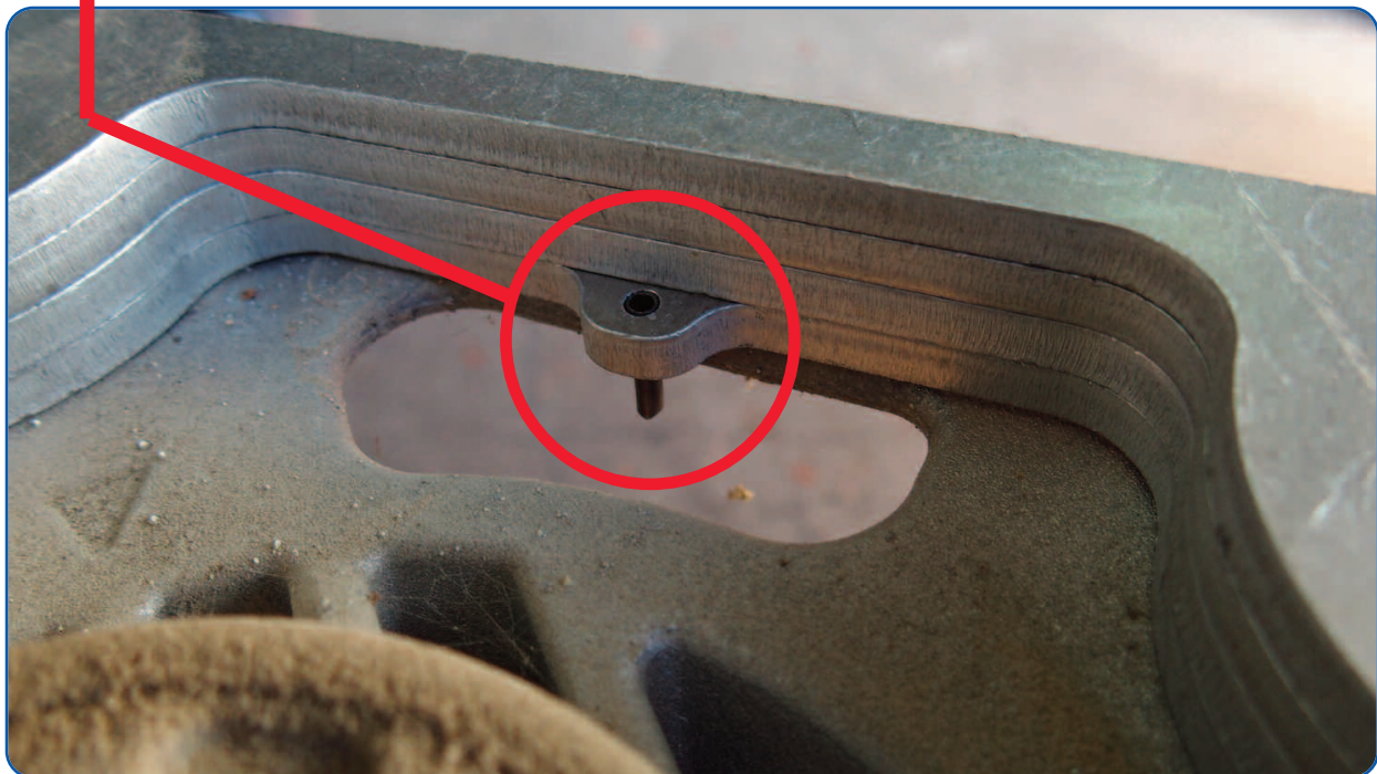
A - Place the thickness of rear shock absorber as shown
