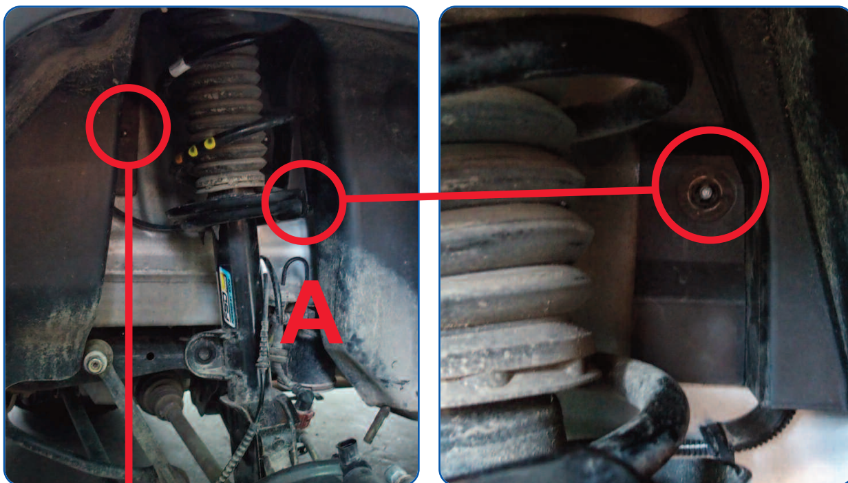
A - Unscrew the two nuts
