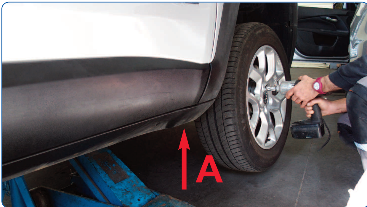
A - Raise the car (axle or crick) and remove 4 wheels
