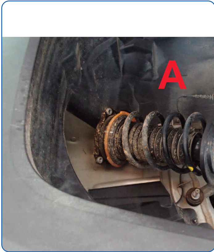
A - Pull out the shock absorber with its spring
