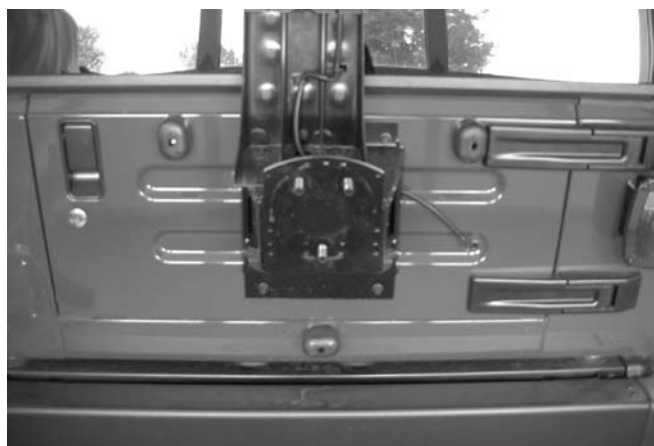
Figure #3 – Remove Spare Tire
